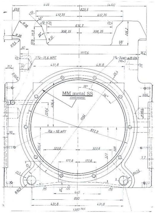
34 damaged back-up rolls bearing houses of a steel work's hot strip mill were modified. The above drawing shows a bearing shell which was damaged by turning of the outer bearing bore. Conventional repairs of these damages would have been executed by welding on, heat-treatening and turning to original size. Cheaper and less time intensive is an innovative repair with MM-metal steelceramic and Hardener yellow.
