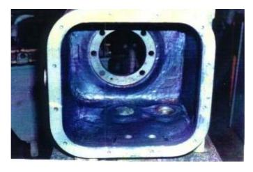
A cracked housing of a hydraulic pump in a steering gear made off aluminium was repaired using MM-metal SS-steelceramic with Hardener yellow. Afterwards the whole housing was coated with VP 10-017 in order to seal the pores in the casting.
