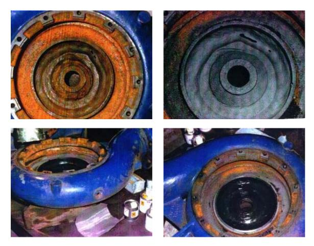
Repair of a pump housing. Damage: erosion and corrosion had reduced the wall thickness to a minimum. The resulting damage was a hole in the housing. For deep wash-outs Ceramium, pasty with MM-Fabric mats (steel) were used. For the purpose of wear-and-tear resistance the pump was coated with Ceramium, liquid.
