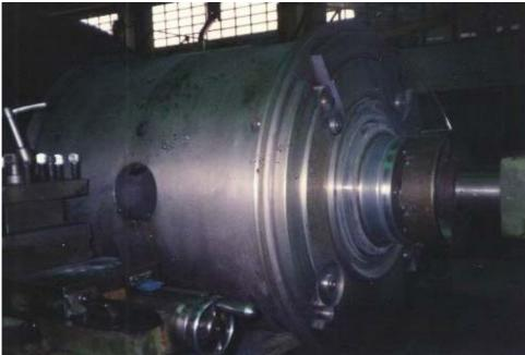
The seat of a ball bearing of a shaft, which serves for lining up, showed an abrasion of 0,2 mm. First the seat of the ball was turned off by 0,5 mm, then the repair site was cleaned with MM-Degreaser Z. Afterwards MM-metal SS-steel with Hardener yellow was applied. Finally the original shaft diameter was reached again by machining. Now the shaft was operational again without any problems.
